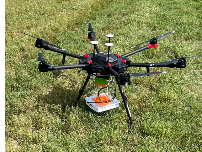
RFID-RM and antenna suspended under the Matrice 600 Pro UAV.
